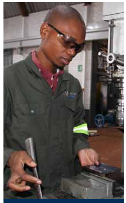
» Calvin Sobopela, Mechanical Fitting Apprentice drilling a hole flange on a drilling machine.
