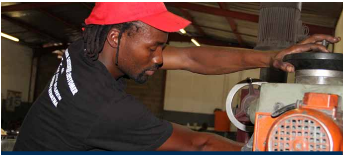
» Xolisa Ngcatsha, an Automotive Machinist Apprentice skimming cylinder heads.
