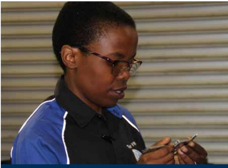
»» Mlilo-Sithole reading measurements after measuring the thickness of brake discs and pads on one of the customer's cars during a routine maintenance.
