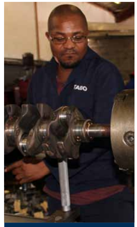
» Tabo Lungisa grinding a crank shaft of an engine.
