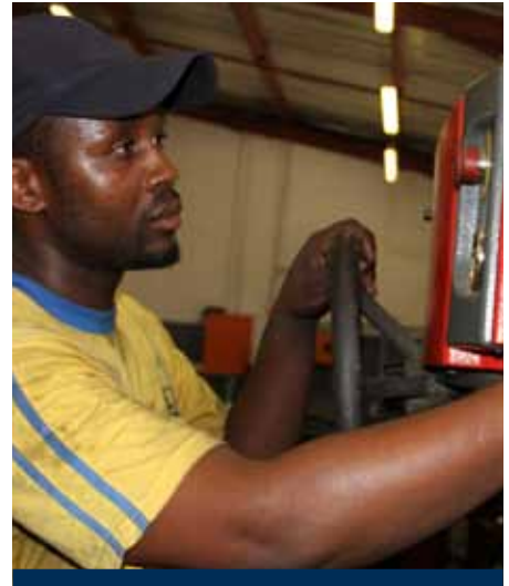
» Sive Gonya, an Automotive Machinist Apprentice grinding seats of cylinder heads.
