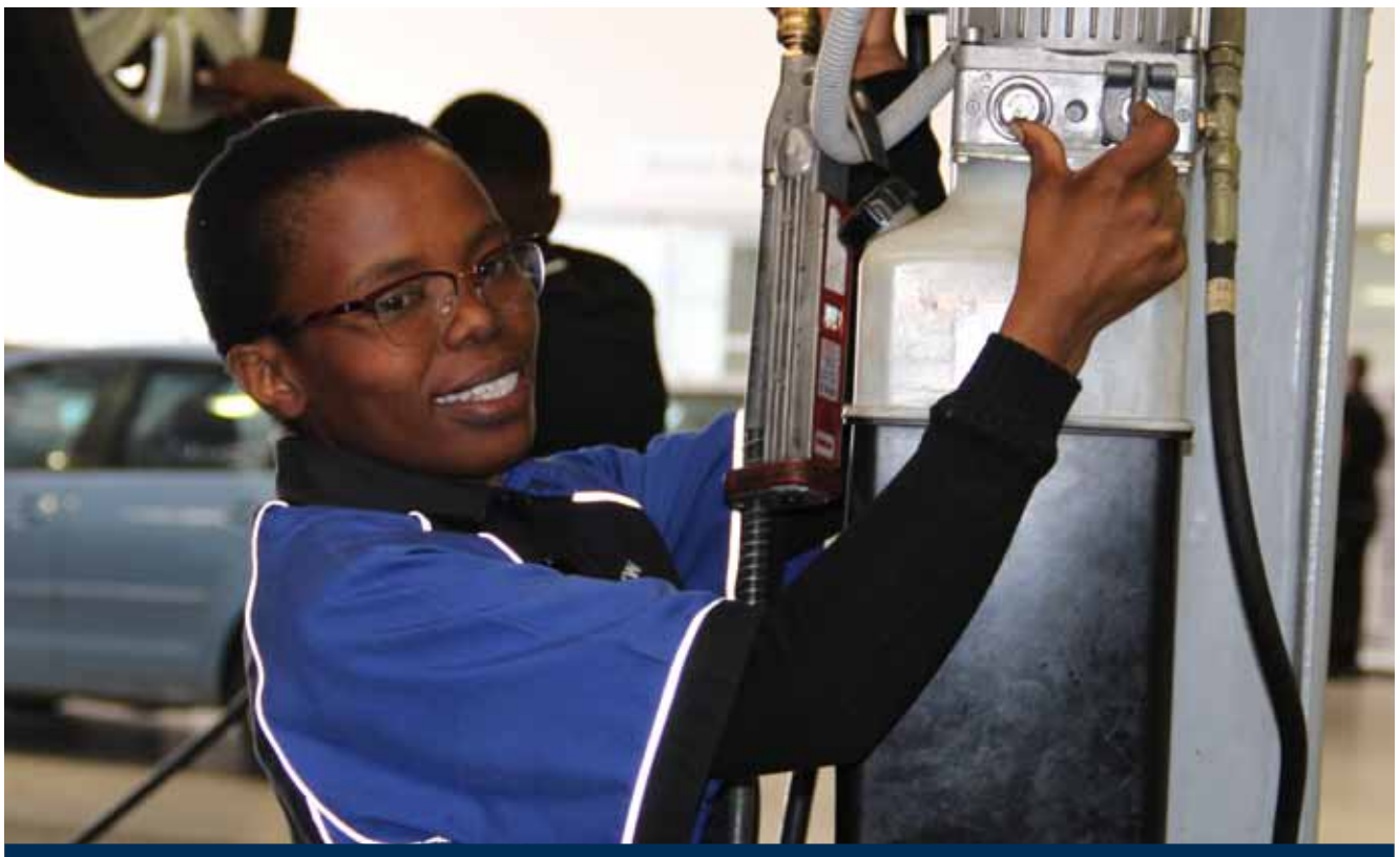
» Mlilo-Sithole lowering the hoist in order to drain and replace oil and oil filter, as well as to replace sump plug during a minor service on one of the customer's cars.
